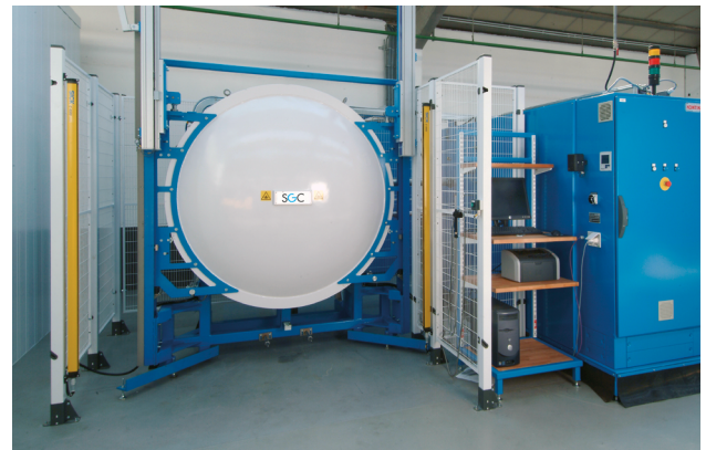
SF 6 filling and sealing station
